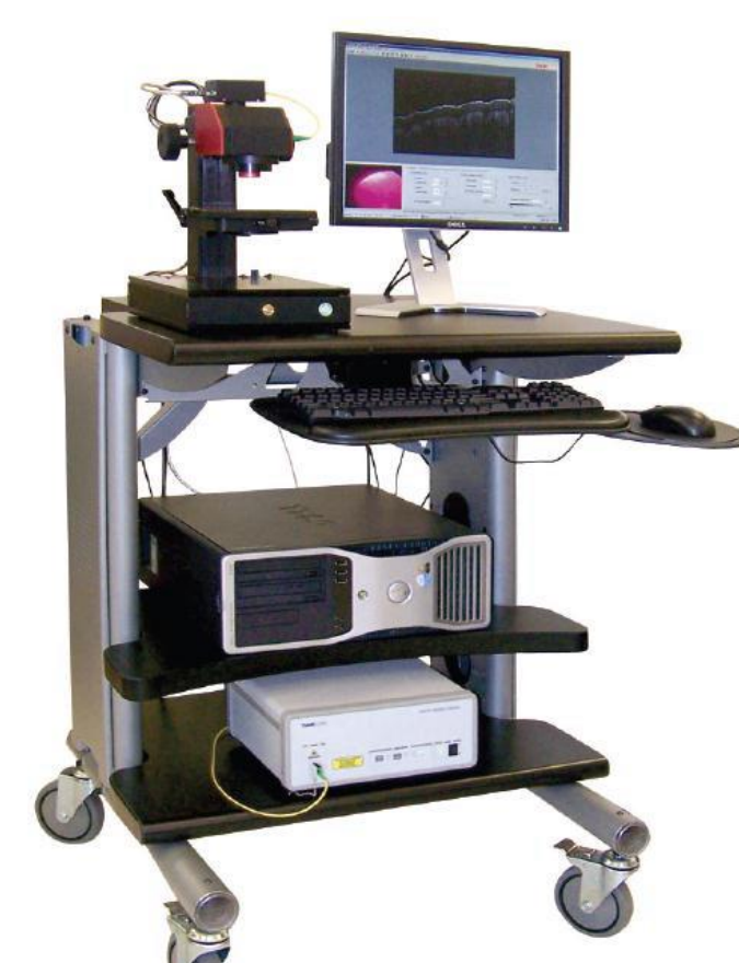
Figure 1: Thorlabs Swept-Source optical coherence tomography imaging system
